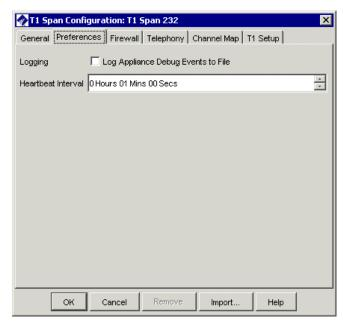
In the Logging area, select the Log Appliance Debug Events to File check box. Clear this check box when you no longer need to store this information, to prevent unnecessary use of hard drive space.
